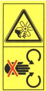
**Hazard: rotating screws – or machine parts!**
